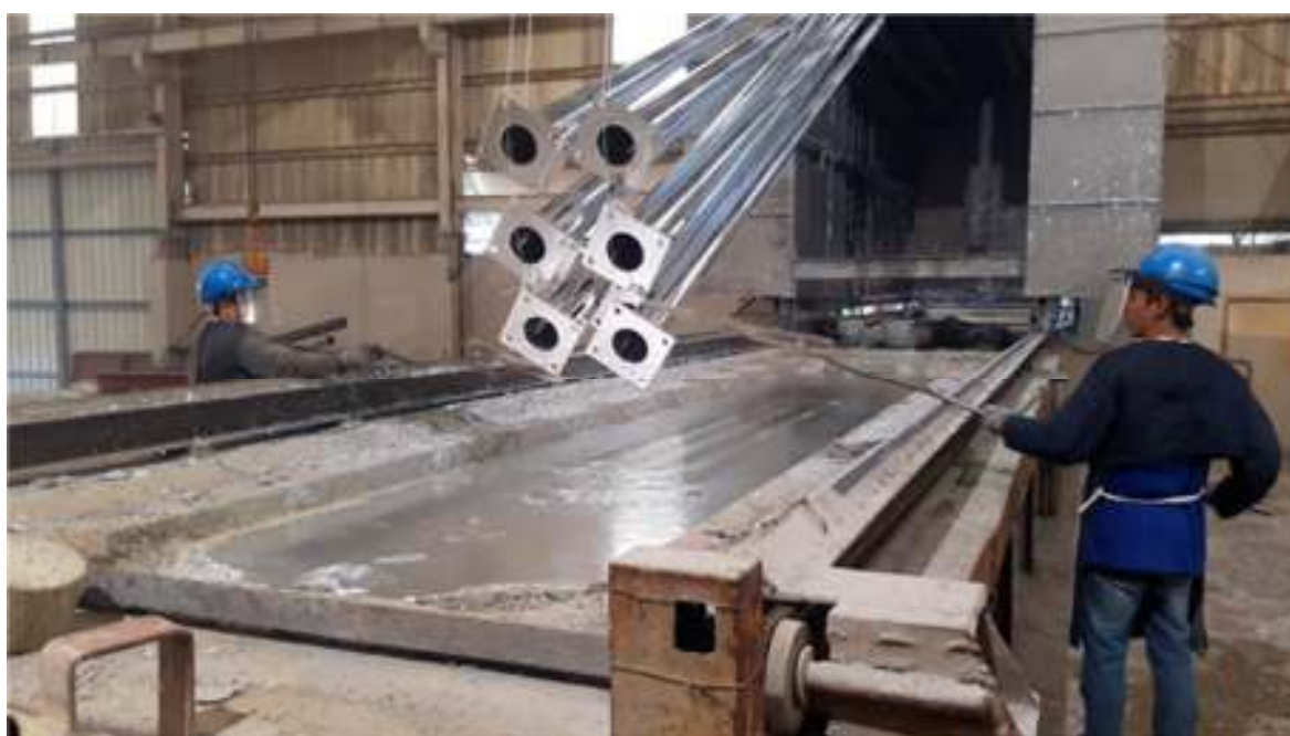
Preparing to hot dip galvanize a batch of steel tubes in a bath of molten zinc
