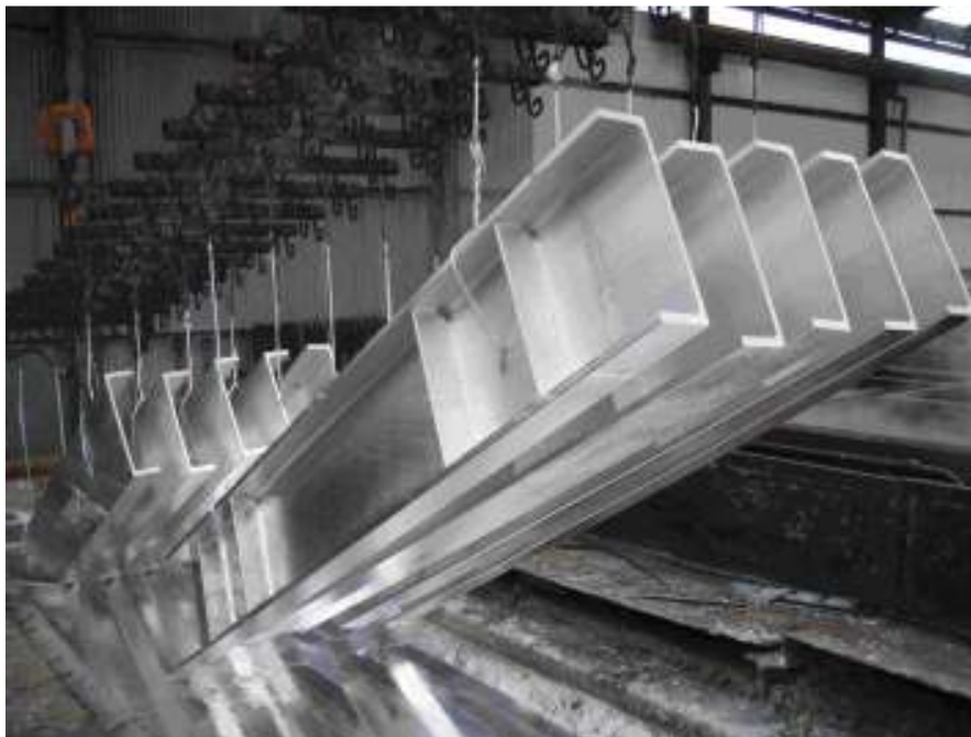
Web forged steel channel products being hot dip galvanized
