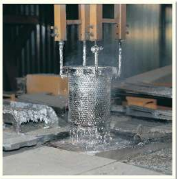
Spin hot dip galvanizing of small components such as nuts, bolts, hinges & fixtures
